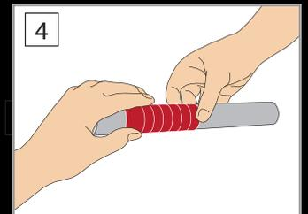
4 To complete wrapping of object, wrap SPITA ResQ-tape completely over previous layer and press firmly.
