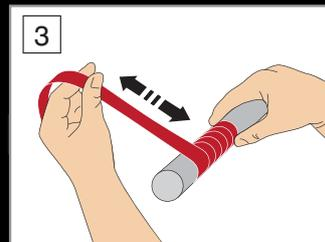
3 While holding SPITA ResQ-tape in place, begin STRETCHING at 3 to 4 times its length and wrap object with 50% overlap to ensure a proper seal.
