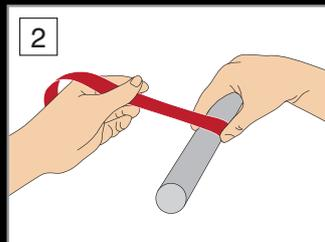
2 Press SPITA ResQ-tape firmly on object being wrapped, hold in place and begin first wrap completely over itself.
